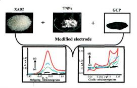
Adsorptive stripping voltammetric determination of imipramine, trimipramine and desipramine employing titanium dioxide nanoparticles and an Amberlite XAD-2 modified glassy carbon paste electrode
