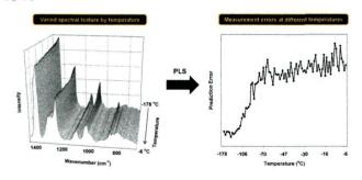
Enhancement of the spectral selectivity of complex samples by measuring them in a frozen state at low temperatures in order to improve accuracy for quantitative analysis. Part II. Determination of viscosity for lube base oils using Raman spectroscopy
