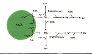
Advanced oxidation using Fe<sub>3</sub>O<sub>4</sub> magnetic nanoparticles and its application in mercury speciation analysis by high performance liquid chromatography-cold vapor generation atomic fluorescence spectrometry
