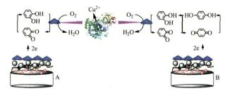
A tyrosinase biosensor based on ordered mesoporous carbon-Au/L-lysine/Au nanoparticles for simultaneous determination of hydroquinone and catechol
