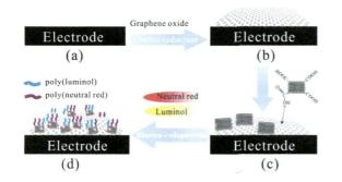
A highly sensitive NADH sensor based on a mycelium-like nanocomposite using graphene oxide and multi-walled carbon nanotubes to co-immobilize poly(luminol) and poly(neutral red) hybrid films
