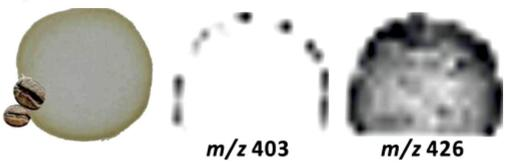
Coffee rings occur during sample preparation for MALDI-MS and LDI-MS.
