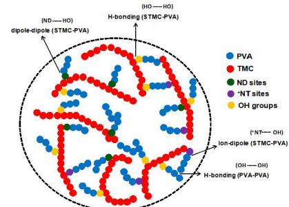
Physical structure of the new copolymers based on *N*-trimethyl chitosan/poly(vinyl alcohol) (TMC-g-PVA) depicting the major interactions that occur among the segments of polymers chains of 6-*O*-succinate-*N*-trimethyl chitosan (STMC) and PVA.
