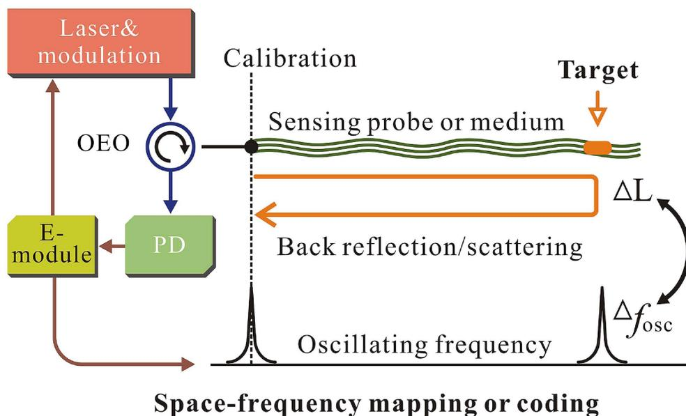
Generic architecture to the OEO-based position-finding approach and the space-frequency coding behind this approach.
