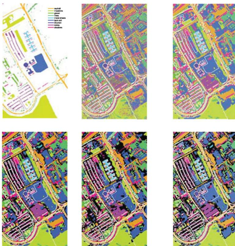
Classification of the Pavia University (Pavia, Italy) scene acquired by the ROSIS sensor: Ground truth (top left) and several classification results with and without context and rejection. For more information, see “Supervised Hyperspectral Image Classification With Rejection,” by Condessa *et al.*, which begins on p. 2321.
