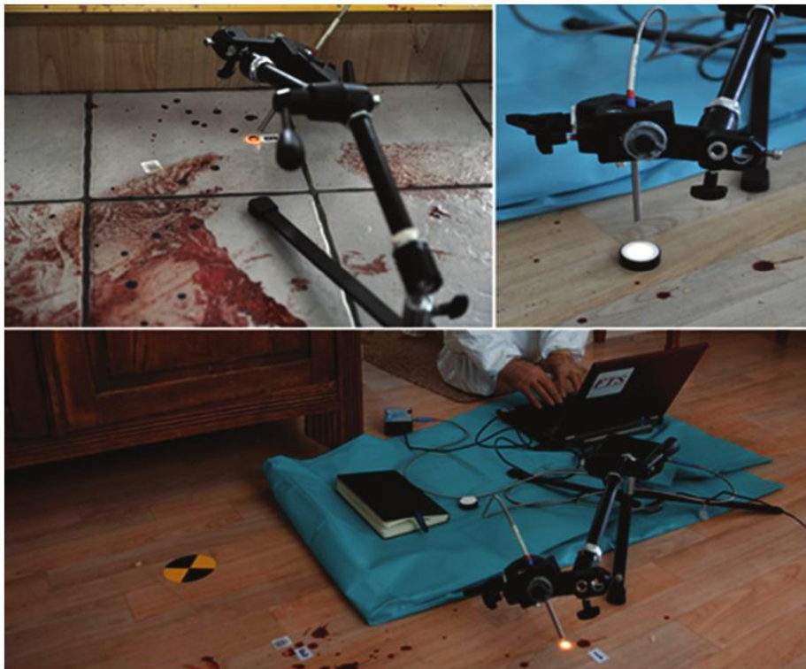
Photographs of the measurement setup used for reflectance measurements of a blood stain (top left), a white reference (top right) and a clean background (bottom) at the crime scene described in "Practical Implementation of Blood Stain Age Estimation Using Spectroscopy" (Gerda J. Edelman et al., article number 0000901)
