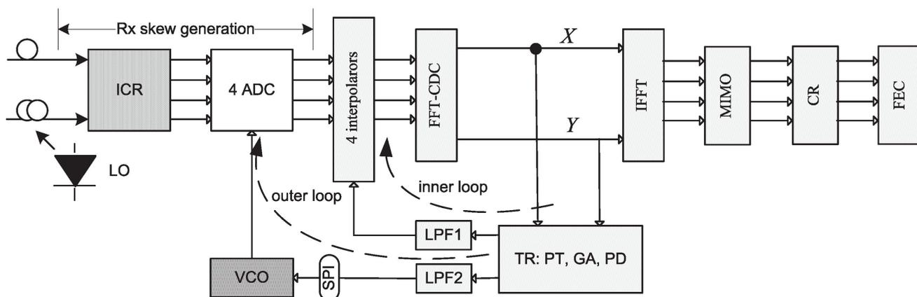
Utilizing digital signal processing to mitigate for skew in photonic components, with the figure above schematically indicating the signal flow for estimation and compensation in the digital coherent receiver, as seen in "An Efficient Method for Skew Estimation and Compensation in Coherent Receivers," by N. Stojanovic and X. Changsong, p. 489.
