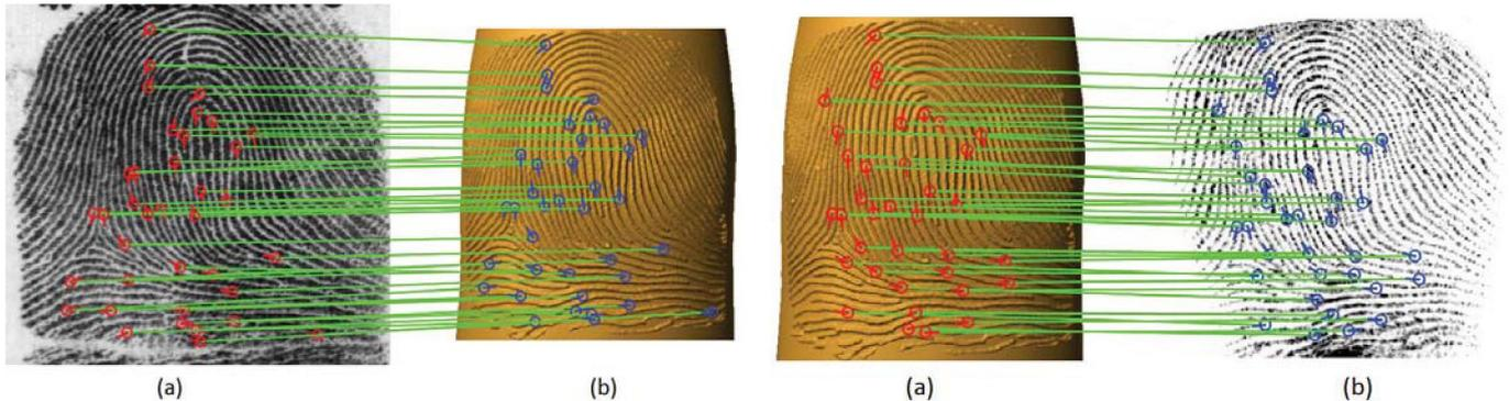
Left: Minutiae correspondence between (a) rolled fingerprint image (S0083 from the NIST SD4), and (b) snapshot of the electronic 3D target generated using (a), as seen in "Design and Fabrication of 3D Fingerprint Targets," by S. S. Arora *et al.*, p. 2284. Right: Minutiae correspondence between (a) snapshot of the electronic 3D target (of fingerprint S0083 in NIST SD4), and (b) the image captured by optical reader 2 (1000 ppi) of the physical 3D target fabricated with FLX 9840-DM.
