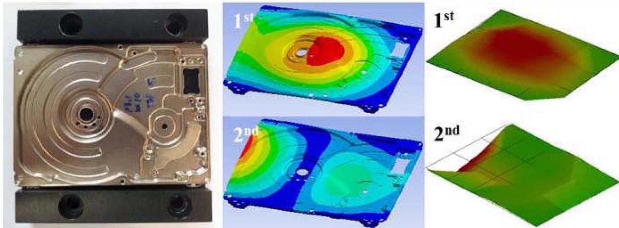
The stamped base and the first and second mode shape, determined from the experiments and simulations. From the paper, “Design Modifications to Improve the Antishock Performance of a Stamped Base for a 2.5-in HDD,” by G. Lim *et al.*, on p. 3301604.
