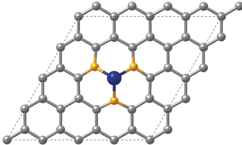
Atomic configuration of Co adatom decorated pyridinic N-doped graphene sheet. Co, N, and C atoms are represented by blue, orange, and gray circles, respectively. From the paper, "Strain-Controllable Magnetism in Co Decorated Pyridinic N-Doped Graphene," by S. Jo *et al.*, on p. 1600104.
