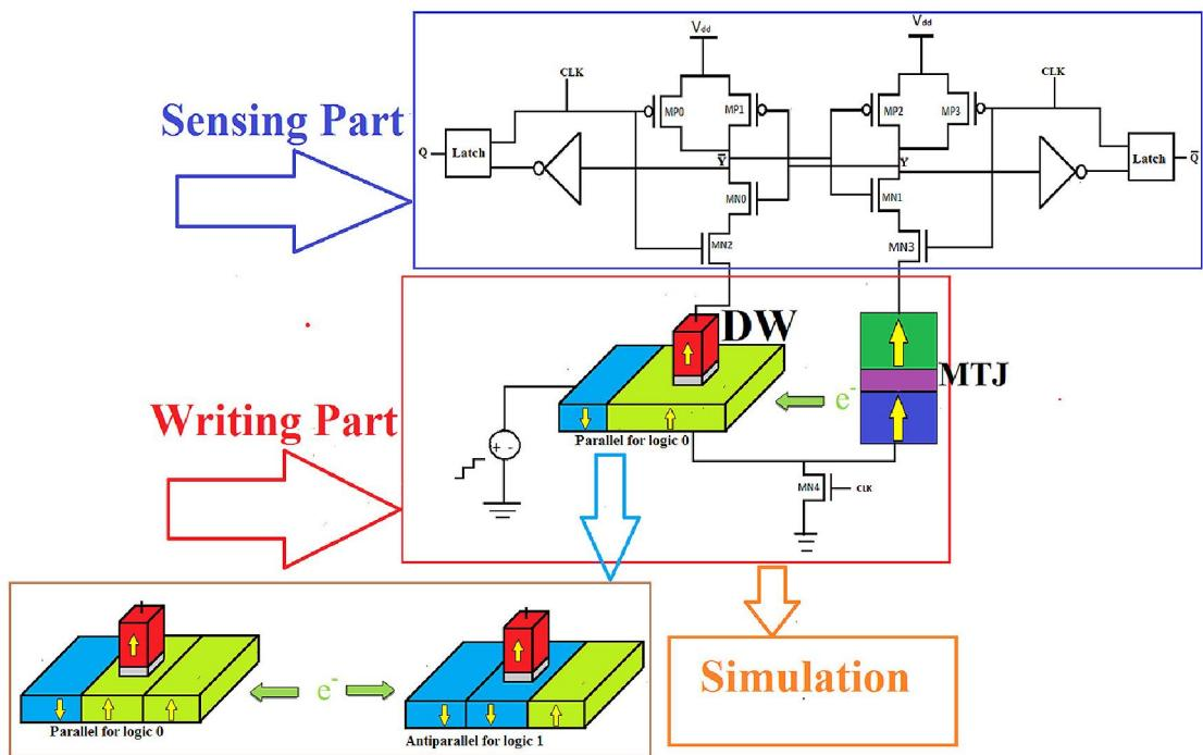
Pre-charge sense amplifier with special magnetic stripe and reference magnetic tunnel junction.
