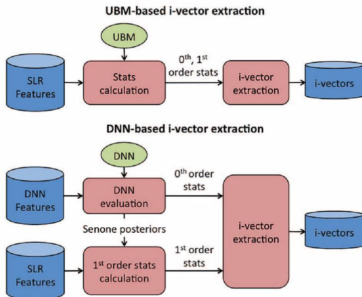
Flow diagram of the GMM-based and the DNN-based i-vector approaches.
