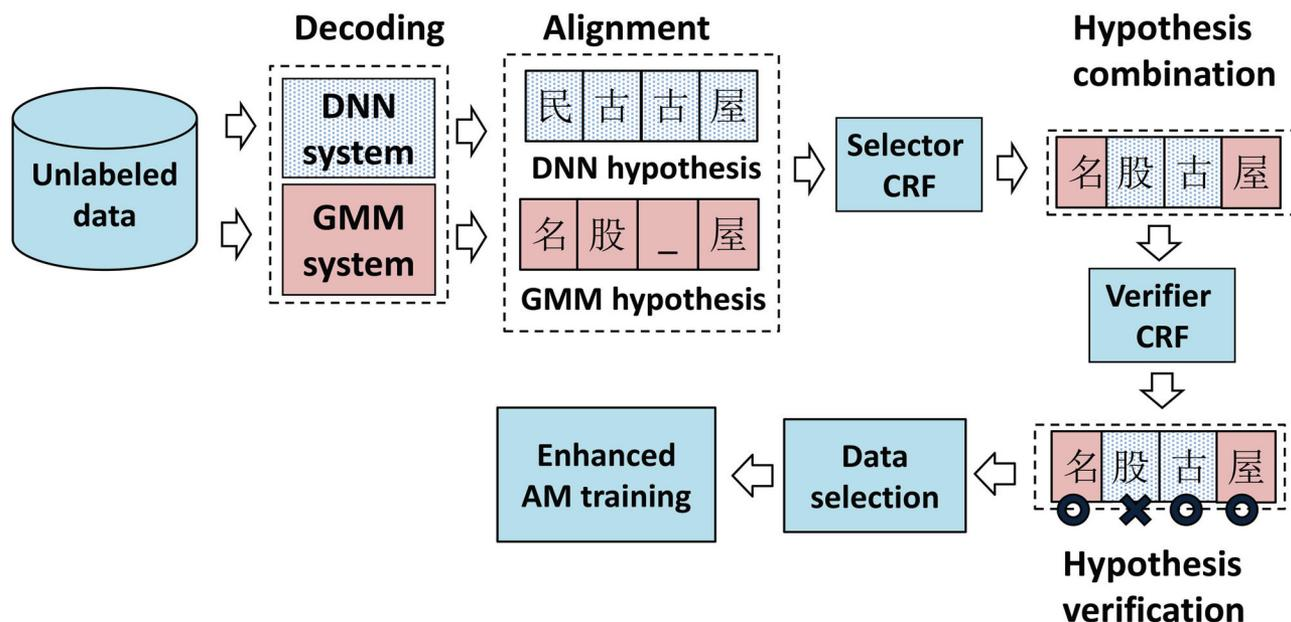
Flowchart of the proposed CRF-based hypothesis combination and data selection method. For more, see "Semi-Supervised Acoustic Model Training by Discriminative Data Selection From Multiple ASR Systems' Hypotheses" by S. Li *et al.*, p. 1524.
