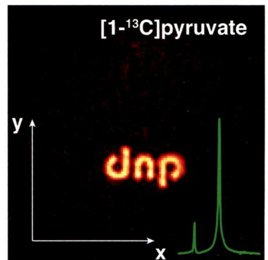
Optimal control derived 2D spatial-selective RF pulses were used in a dissolution DNP and MRI setup to localize  $^{13}\text{C}$  signal in hyperpolarized pyruvate samples.
