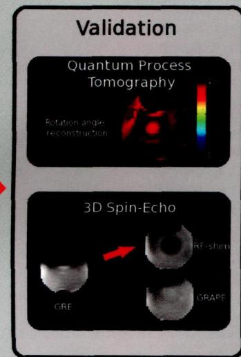
After measuring B0 and B1 maps of a parallel transmission setup (left), ultra-high-field data is fed into a gradient ascent pulse engineering program to design refocusing, B1 inhomogeneity-mitigating pulses (middle). Spin-echo MRI and quantum process tomography experiments (right) validate these quantum control tools.
