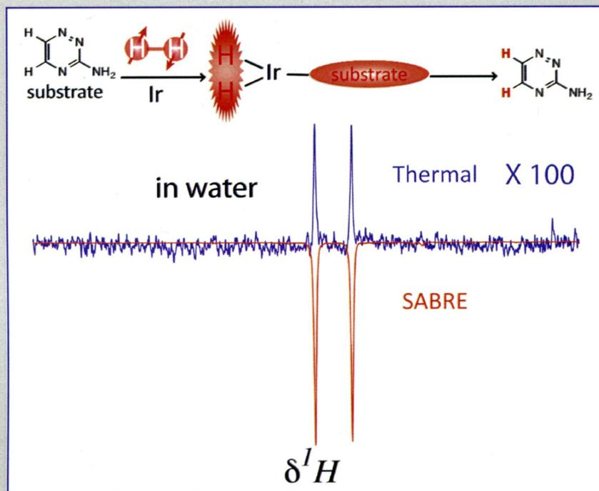
Signal Amplification By Reversible Exchange (SABRE) parahydrogen polarization of 3-amino-1,2,4-triazine in an aqueous mixture, delivers 1% polarizations in less than 1 min.
