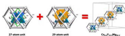
Reported is the Mg-rich intermetallic compounds Y 5-x Mg 24+x series adopting the cubic α-Mn type structure and its complex ternary derivative Ce 6.9 Y 12.5 Mg 92.2 crystallized in a defect Sm 11 Cd 45 type structure with a nearly twice larger lattice parameter than those of the Y 5-x Mg 24+x series. Electronic structure calculations show nearly free electron like behavior, but with a distinctive pseudogap in the density of states curve for the ternary system.
