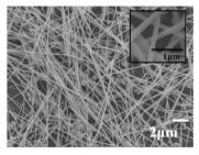
The FE-SEM image shows that nanostructures with considerable quantities of silver nanowires can also be produced when the PVP  $(Mw=360\ K)/AgNO_3$  molar ratio was 2.5.
