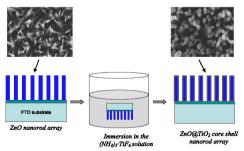
The synthesis process of coating  $\rm TiO_2$  shell onto ZnO nanorod core is shown schematically. A thin, uniform, and conformal shell had been grown on the surface of the ZnO core after immersing in the  $\rm (NH_4)_2$ : $\rm TiF_6$  solution for 5–15 min.
