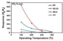
The response of 0.25 wt% Pt-loaded WO $_3$  sensor was 637 towards NO $_2$  concentration of 10 ppm at 150 °C.
