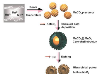
The MnO 2 shell with MnCO 3 intermediate core is prepared at room temperature; the hollow structure with excellent permeated shell enhanced the discharge capacity and electrochemical stability.
