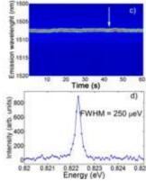
The emission linewidth is a key figure of merit for a quantum emitter. This paper reports on the possibility of reducing the spectral linewidth of single-wall carbon nanotubes. It demonstrates an order of magnitude narrower linewidths compared to the available data due to the enhanced crystalline quality of the carbon nanotubes synthesized by using a laser ablation technique.
