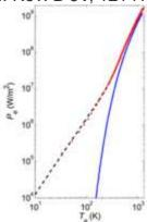
The electron-phonon scattering dominated heat dissipation is difficult to observe in graphene due to the role of impurities in scattering processes. Owing to the suppression of flexural-mode-induced supercollisions in suspended bilayer graphene, the authors of this paper are able to demonstrate that the intrinsic electron-optical phonon coupling governs the heat flow in suspended bilayer graphene samples.
