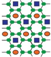
Density functional theory calculations of the electronic properties of graphene-hexagonal indium telluride superlattices predicts two inequivalent geometrical structures that are almost degenerate in energy. These structures give rise to either gapped states in Kekule phase or gapless states in reconstructed graphene Dirac cones. The results of this study will be useful for exploring the possibility of many-body instabilities in two-dimensional systems.
