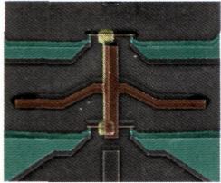
Normal state copper island connected by insulating aluminum oxide tunnel barriers to a pair of superconducting aluminum leads. [Ville F. Maisi et al. , Phys. Rev. Lett. 112 , 036801 (2014)]
