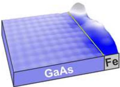
The electronic charge distribution at the iron/gallium interface is imaged directly with high spatial and energetic resolution. The metal-semiconductor electronic barrier properties are found to be dependent on both the charge distribution and chemical bonds between the metal and semiconductor atoms.
