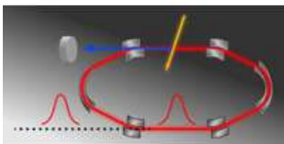
A cooled ring stores high-speed negative ions for more than 1000 seconds and enables new studies of atomic and molecular ions that are important in interstellar and atmospheric chemistry.
