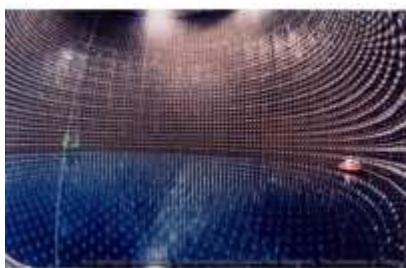
Super-Kamiokande's 22.6 kton cylindrical water Cherenkov detector has provided the most stringent upper limit on the proton-WIMP dark matter scattering cross section.
