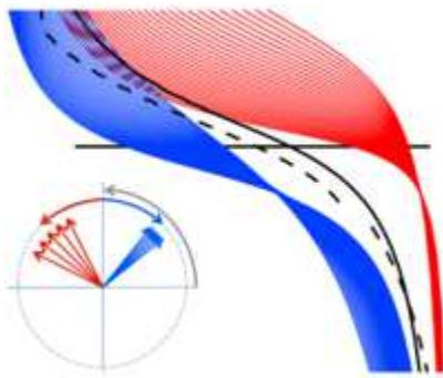
Light-induced shifts in atom interference fringes are shown to be significantly affected by the Earth's rotation rate, opening the door to a new type of atom interferometer.
