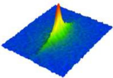
An optical dipole field is used as a collimating lens to cool Rubidium atoms to record-low kinetic temperatures of 50 picokelvin.
