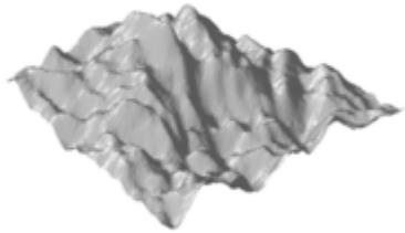
Experimental water tank measurements of gravity-capillary surface waves show 3-wave coupling is important in the build up of water wave turbulence.
