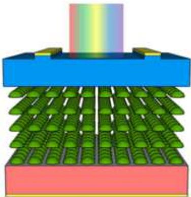
The spectral range over which intermediate band gap solar cell devices absorb is significantly increased, with absorption for wavelengths from 250 nm to 6000 nm. In these materials a photocurrent is produced when the material is irradiated with photons with energies below the bandgap of the material.
