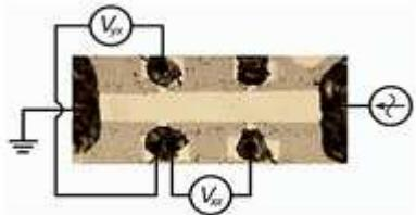
Thin films of magnetic topological insulators can exhibit a nearly ideal quantum Hall effect without requiring an applied magnetic field.
