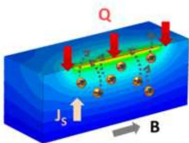
A spin current is experimentally generated in various insulating paramagnets using thermal gradients, a surprising result as, unlike ferromagnetic insulators, paramagnets do not hold their magnetization when the applied field is removed.
