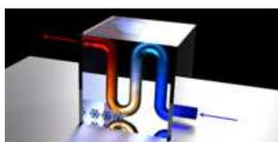
A gas of polaritons can serve as a coolant fluid that transports heat away from a semiconductor microcavity.
