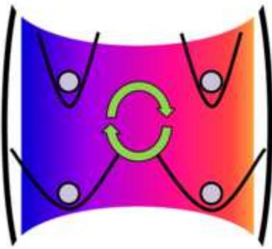
A nanoparticle levitated in an optical cavity is proposed as a Stirling type heat engine – where the particle is driven through a cooling-heating sequence that changes the mechanical oscillations of the systems and generates heat.
