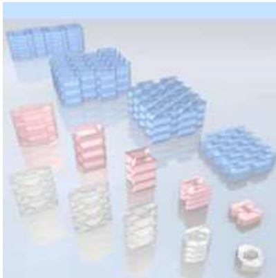
Structures made solely from folded rigid planes exhibit both tunable negative Poisson's ratio and structural bistability allowing for the construction of new types of mechanical metamaterials.
