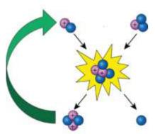
Alpha particles would need to provide 50 kJ of heating to achieve a burning plasma regime - where more energy is released by the fusion reactions than is absorbed by the fuel - at the National Ignition Facility.
