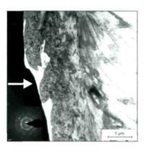
Sand castings produced of steel GX25CrMnN18-18 with ~0.6 mass% N reached a proof strength  $R_{\rm p0.2}$ = 457 MPa and a reduction of area Z = 60%. The resistance to pitting corrosion was better than that of steel X5CrNi18-10 and the resistance to impact wear equal to that of Hadfield manganese steel. An amorphous and nanocrystalline layer is formed in the wear surface.
