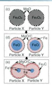
If being coated with MgO, magnetite particles will not sticking each other when they are reduced to the same metallization rate in fluidized bed with CO–H<sub>2</sub> mixtures as that of sticking particles without coating. Because coating MgO can not only decrease the chance of touch between metallic iron on the surface of different particles, but also provides the action time for carbon deposition and the production of Fe<sub>3</sub>C with low viscosity.
