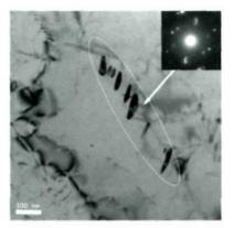
After the normalizing and tempering, simulated post-welding heat treatment and step cooling, the carbide precipitates of the ferritic heat-resistant steel 2.25Cr–1Mo evolve from M<sub>3</sub>C to M<sub>7</sub>C<sub>3</sub> and M<sub>23</sub>C<sub>6</sub>. The coarsening of carbides deteriorates impact toughness, and the morphology, crystal structure, and chemical composition of carbides are also important influencing factors.
