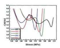
The formation of ferrite during rolling at temperatures above the Ae<sub>3</sub> is a controversial topic. Here it is shown that strong evidence for the occurrence of this transformation can be obtained directly from the flow curve of the deformation using the double-differentiation method. The critical strain for dynamic transformation is shown to be distinctly less than that for dynamic recrystallization.
