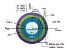
A new double calcium treatment method is proposed according to industrial experiment. In the new process, the evolution of inclusion is analyzed and the controlling standard of T.[Ca]/T.[O] ratio for calcium treatment is discussed. In order to get a good calcium treatment result, T.[Ca]/T.[O] ratio should be controlled above 0.91, and the ratio between 0.91 and 1.25 is suitable in present work.
