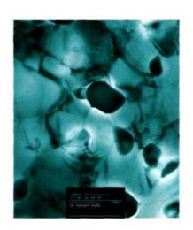
In this work, thermodynamical equilibria have been calculated for super hard high speed steel, AISI M41 composition belonging to the multicomponent system Fe-C-Cr-W-Mo-V-Co as well as for its three different variants containing niobium. Effect of niobium and high cooling rate during electroslag remelting on the precipitated carbides, morphology of carbides, secondary hardening temperature, and wear rate of investigated steels are studied.
