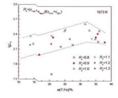
The partition ratios of phosphorous between  $CaO-SiO_2-Fe_1O-P_2O_5$  slag with  $Na_2O$  or  $K_2O$  addition and solid pure iron are measured at different temperatures to learn about those between the same slag and carbon-saturated iron. The experimental results shows that both  $Na_2O$  and  $K_2O$  addition can improve the dephosphorization ability of the experimental slag and they have similar dephosphorization ability under the same experimental conditions.
