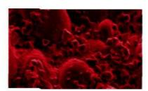
Leaching of chromium from the slag deposits is a major environmental problem that needs serious attention. Chromium in slag if not stabilized in spinel phase, could oxidize to Cr<sup>6+</sup>, and leach out by rain water. In the current work, the effect of alumina addition on chromium partition in slags been studied under the conditions close to the industrial. The results presented can reveal how to optimize spinel phase precipitation.
