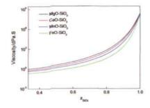
A structurally based model is developed to calculate the viscosity of aluminosilicate melts by composition and temperature. According to the comparisons with other viscosity models, better estimation results can be obtained by the present model for both quinary, quarternary, ternary, binary, and unary systems involving MgO, CaO, FeO, MnO, Al<sub>2</sub>O<sub>3</sub>, SiO<sub>2</sub> components.
