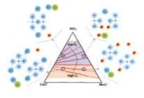
The sulphide capacities of the CaO−SiO₂−MnO(−Al₂O₃−MgO) slags are measured at 1873 K using a gas–slag equilibration method. The effects of MnO and the MnO↔CaO substitution on the sulphide capacity of molten slag are also investigated based on the structural view of silicate melts. The dissolution mechanism of sulphur in Ca−Mn–silicate melts can be explained by the "Competitive dissolution mechanism."
