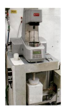
Based on known calibration problems with high-temperature measurements, the viscosity is calculated directly without calibration. This is possible with an air-bearing rheometer and exact absolute torque measurement via the electrical parameters of the drive and via movement parameters and geometry. This technique meets the desired requirements in view of measuring accuracy and reproducibility.
