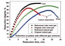
The utilization of coke oven gas for production of DRI in the integrated steelmaking route is considered as an efficient method to maximize the efficiency of the process. In this study, pellets are isothermally reduced with simulated original and reformed coke oven gas at 700-980°C. The results are compared with those obtained by the reduction of pellets with natural gas.
