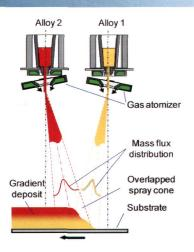
This paper describes a newly developed spray forming process for the manufacture of graded materials. In this process, two different tool steels are atomized simultaneously and co-sprayed on a flat substrate, resulting in a flat graded deposit when the two sprays are overlapped. By the use of the new co-spray forming process, different microstructures and properties can be combined in a single deposit.
