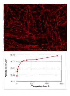
The coarsening rate of carbide particles at 800°C is determined experimentally and calculated. By substituting in LSW equation molar carbide content with atom content of chromium in solid solution, the difference of both rates is lower by 2 orders of magnitude. It is confirmed that the smaller difference is due to the shorter diffusion time for chromium atoms from solid solution than from decomposing carbide particles.
