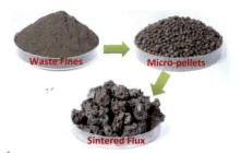
Mixture of waste iron oxide fines and lime fines are micro-pelletized without binder using CO<sub>2</sub>/industrial waste gas at room temperature that can provide a good handling strength. Subsequently, the developed micro-pellets are sintered without using coke breeze. Waste materials itself provides heat for sintering. The produced sinter would be useful as a synthetic flux in basic oxygen process for early formation of oxidizing slag to make refining faster.
