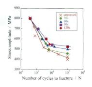
Shot peening using conventional cast steel shots is conducted for the purpose of improving the fatigue characteristics of spring steel. To examine the effect of shot peening on fatigue strength, fatigue tests are carried out in a plane-bending test machine. It is found that the fullcoverage time, 90 s, is required in order to improve the fatigue life.
