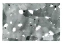
The effects of copper on mechanical, microstructural, and recrystallization behavior are investigated. As-cast microstructure mainly consists of polygonal ferrite and Widmanstatten ferrite. It is found that copper increases strength and hardness by solid solution strengthening and precipitation hardening in as-cast condition. Recrystallization responses are strongly dependent on initial microstructure and Cu content.
