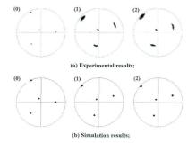
The deformation behavior and orientation development of two copper single crystals with symmetrical orientation to the ideal shear plane during ECAP process have been successfully studied by crystal plasticity finite element method model. The significantly influence on the corner gap formation and morphology of plastic deformation zone has been observed. Simulation results agree well with the earlier published experimental measurements.
