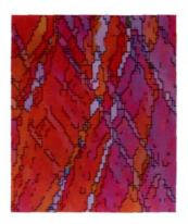
Copious recrystallization occurs in some deform grains during the early stages of annealing in an automobile body making steel. In this article the origin of the event is explained by characterizing the deformation microstructures with electron backscatter diffraction technique. The intersecting micro-shear band locations comprise all necessary elements to operate as fast acting recrystallization sites.
