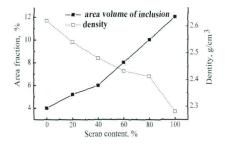
The influences of casting parameters and inclusions on the hydrogen content is very useful in situ aluminum alloy casting procedure to control the hydrogen content. The hot alkaline deep etching method can evaluate the area fraction of the oxide inclusions in aluminum alloy successfully, and provide a convenient and effective method in situ production for inclusion detection.
