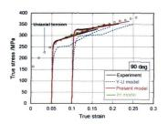
Stress-strain responses of IF sheet metal under uniaxial tension in the 90° after uniaxial pre straining. The Modified Yoshida-Uemori model shows a good agreement with the corresponding experimental stress strain responses.
