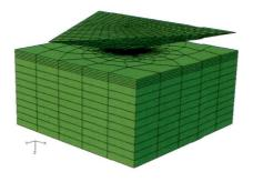
A crystal plasticity finite element method model has been developed to investigate the effect of the initial orientation on the surface profile patterns of aluminum single crystal during nano-indentation. This 3D model has been validated by comparison with experimental observations. The slip traces are analyzed to provide detailed explanations of the anisotropy of the piling-up patterns.
