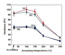
Upon annealing at 100°C for 30 min, hardening by annealing occurrs for all the ARB deformed materials, although the increment for AA6061 is larger [curve (a) and (b)] than AA1050 [curve (c) and (d)]. Slight softening is observed after annealing at 150°C. However, the decrement in hardness is not obvious until annealing at 200°C and above.
