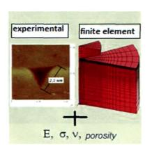
This paper describes a combined FE simulations and nanoindentation experiments to obtain the depth dependent mechanical properties of oxide layers on high speed steels (HSS). The interaction between the mechanical properties and nanoindentation parameters such as the maximum load and unloading slope of the load-displacement curves are established via multiple regression analysis.
