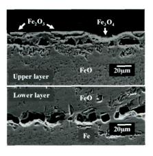
Oxidation behavior of low carbon steel is investigated in oxygen and water vapor using continuous thermogravimetric analysis (TGA). The effect of temperature, oxygen pressure, and water vapor content on the oxidation of the steel is studied. The morphology, composition, and microstructure of oxides formed in moist atmosphere are examined and analyzed by X-ray diffraction (XRD), scanning electron microscope (SEM), and energy dispersive X-ray analysis (EDX).
