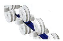
The knowledge of the loads occurring in the roll forming process is important for the design and dimensioning of the process. One option to detect these loads provides the simulation. Due to simplifications in the used simulation model and the unknown interactions between sheet metal and roll forming machine, important parameters, such as contact normal pressure cannot be displayed realistically. This paper shows a way to quantify these variables in the simulation.
