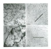
The comprehensive property of Nb-bearing pipe line steel processed with ultrafast cooling is corporately improved through dislocation and precipitation strengthening, while the matrix microstructures are mostly massive ferrite characterized by sharpedged curved grain boundary.
