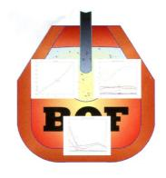
In order to validate the BOF process model, the heats in 170- and 330-ton converters are simulated. The behaviors of the metal and slag phase components, temperature and charge material melting, and dissolution are shown and analyzed. Using the simulation results, the oxidation–reduction behavior of phosphorus and manganese during the converter steelmaking process is explained.
