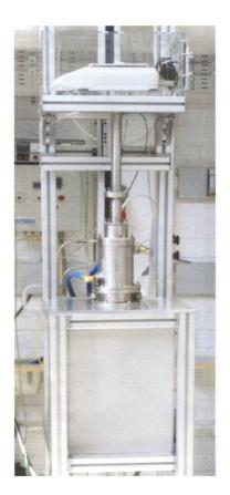
A new TG setup has been developed to study reactions involving weight changes (even solid–solid reactions). The advantage of this method over the conventional TGA is that it avoids the gradual change of gas composition in the initial stages. The setup has been used to study reduction of hematite pellets. Reduction rates obtained have been found considerably higher than the conventional TG.
