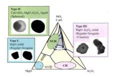
Characteristics of non-metallic inclusions are investigated in high Si-containing (1.9 and 2.7% Si) stainless steel grades with respect to clogging problems during casting. The obtained results and thermodynamic calculations using Thermo-Calc and FactSage show that the main reason of clogging during casting of these steels having larger than 0.003% of Al is relatively high contents of spinel MgO-Al<sub>2</sub>O<sub>2</sub> inclusions and clusters in liquid steel.
