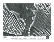
Reverse transformation from a ferrite/pearlite to austenite is investigated in spring steel 60Si2MnA with various pearlite fineness obtained by isothermal transformation. Effects of heating temperature, holding time and interlamellar spacing on the reverse transformation are analyzed and the mechanism of the structure inheritance in the spring steel during heat treatment process is discussed.
