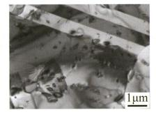
The austenite phase of duplex stainless steels (DSSs) is always considered to undergo nearly no phase transformation or precipitation upon annealing. The ferrite phase, on the other hand, is always regarded as the active transforming/precipitating phase. However, it's been found that if DSSs are plastically deformation and annealed between 900 and 1050°C, then the situation will be totally opposite.
