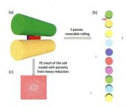
In this paper, a two-step strategy is preceded using THERCAST3D to obtain the information of solidification firstly. Then, a software FORGE3D is used to simulate the heavy reduction and ultra-heavy plates rolling. The aim is to find out the closing behavior of porosity voids in slabs in the process of heavy reduction combined with low compression ratio rolling.
