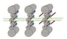
A roll-strip-tension coupling model with both accuracy and efficiency is established for cold rolling process with tension. Then the self-correction effect of front tension and the attenuation effect of back tension on flatness deviation are analyzed by the calculation results of the model, and corresponding quantitative correction coefficient and attenuation coefficient are obtained.
