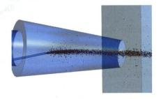
Auxiliary fuel injection into the blast furnace has many benefits in blast furnace operation. Increase of oil injection levels has proven challenging. CFD model is developed to study injection of heavy oil in terms of atomization and mixing. Properly designed nozzle is shown to improve mixing significantly allowing higher injection levels.
