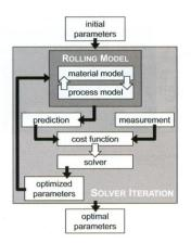
The aim of this paper is to obtain valid material parameters for semi-empirical material models directly from industrial rolling operations. The principle idea here is to use inverse modeling techniques. Sound roll force predictions thus can be enabled without conducting time and cost intensive laboratory tests. The validity of the proposed concept is demonstrated using demanding test cases.
