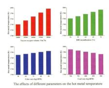
A calculation model has been developed to study the relationship between parameters and hot metal temperature. The results show that for every 10K increase in hot metal temperature, the tuyere oxygen volume, metallization, fuel rate, and coke rate should increase by 714.3 m<sup>3</sup>h<sup>-1</sup>, 6.4%, 90.9 kg tHM<sup>-1</sup>, and 29.4 kg tHM<sup>-1</sup>, respectively, while the coal rate should decrease by 115.7 kg tHM<sup>-1</sup>.
