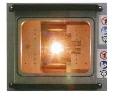
The strength of metallurgical coke is vital for efficient blast furnace operation. The hot strength of industrial cokes is studied by using a Gleeble 3800 thermomechanical simulator. The properties of coke that could affect their hot strength are determined and discussed.
