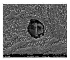
SEM analysis is involved in studying ductile fracture mechanism in upper and lower bainitic steels. Detailed microstructural analysis reveales that cracking and interface decohesion of Al<sub>2</sub>O<sub>3</sub> inclusions at lower strains and decohesion of cementite/ ferrite matrix interfaces at higher strains are the main void nucleation mechanisms. Void growth behavior is also modeled. Moreover, final fracture mechanisms are examined and cleared in both steels studied.
